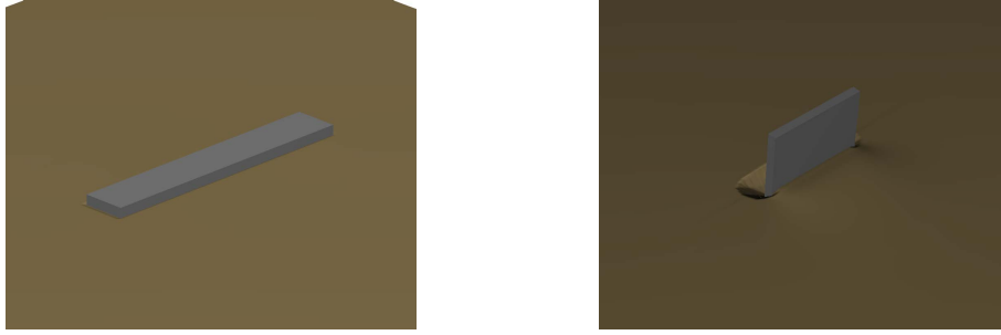
Fig. 6: Overview on the scenarios used to validate the soil flow in SCM against. Strip load experiment on the left and the blade experiment on the right.
