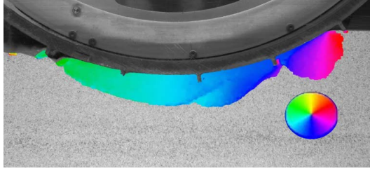
Fig. 3: Particle image velocimetry (PIV) [13, 14] used as reference during the development of new algorithm. PIV images provided by NASA/JPL/Carnegie Mellon University.
