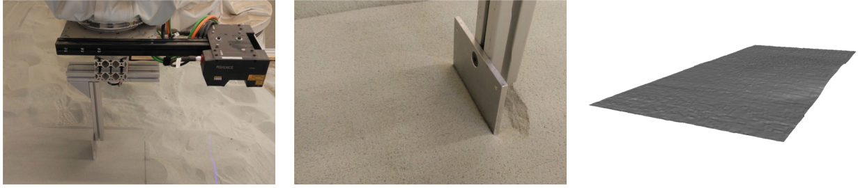
Fig. 8: Experiment to determine the parameters \Psi_{\text{Angle}} and \Psi_{\text{Distance}} using the TROLL [4]. General experiment setup shown on the left, the resulting deformation shown in the middle and the surface scan of the resulting deformation on the right
