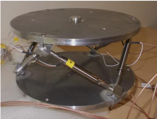
Fig. 7: Preliminary version of absorber with piezo-actuators
