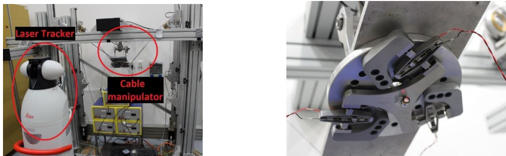
a) end-effector position feedback using laser tracker b) end-effector attached to the cable structure using piezo actuators
