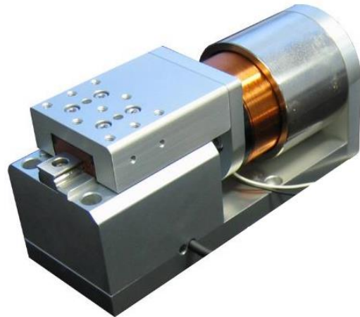
Fig. 8: Voice-Coil actuator chosen for future prepared experiments
