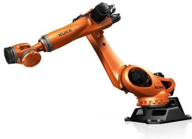
b) Serial robot manipulator with 6 rotational constraints
