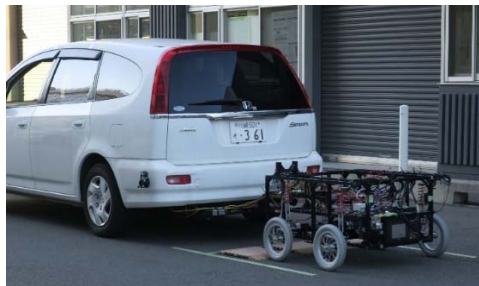
Fig. 2: Experimental trailer for road profile measurement
